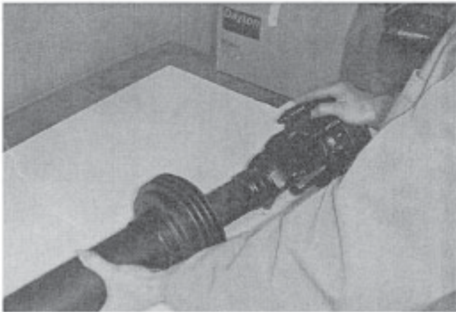
Figure 16) Grasp the Yoke and shield tube and pull shaft from the shield.
